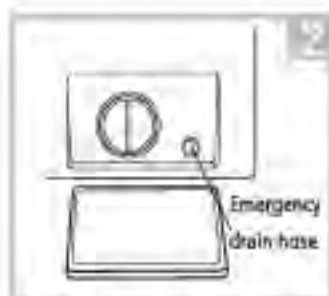
Rotate 90°C and pull out the emergency drain hose, and take off the hose cap
