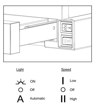
To achieve better extraction, we recommend switching on the extractor a few minutes before starting to cook (3—5 minutes) so that the air flow is continuous and stable when extracting fumes.
