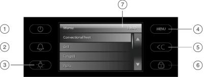
The appliance is operated via the display (7) and the electronic sensors next to and below the display. These react to finger contact. An audible tone will sound each time a sensor is touched. The volume of the keypad tone can be adjusted or switched off altogether, see "Setting-Volume-Keypad tone".
