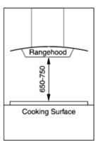
Install Range Hoods in accordance with the manufacturer's instructions. Technika recommends that all Range Hood clearances be a minimum of 650mm to a maximum of 750mm (between the top of the cooking surface and to the underside of the rangehood).
