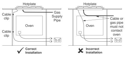
Replacing the power supply lead
