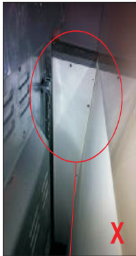
Left Side of oven, chain not attached
