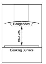
Install Range Hoods in accordance with the manufacturer's instructions. Technika recommends that all Range Hood clearances be a minimum of 650mm to a maximum of 750mm (between the top of the cooking surface and to the underside of the rangehood).
