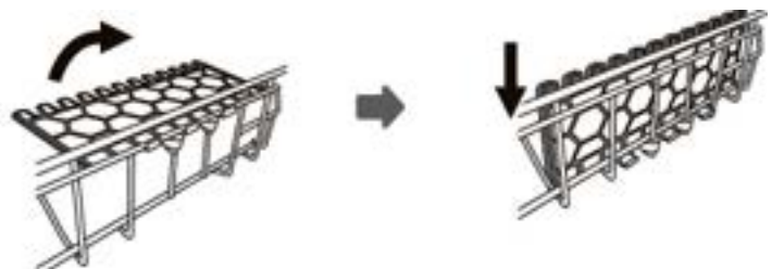
1 To raise the upper basket, just lift the upper basket at the center of each side until the basket locks into place in the upper position. It is not necessary to lift the adjuster handle.
