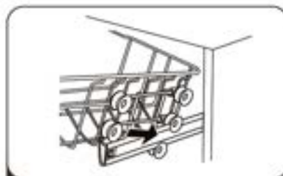
3 Re-attach the upper basket to upper or lower rollers.
