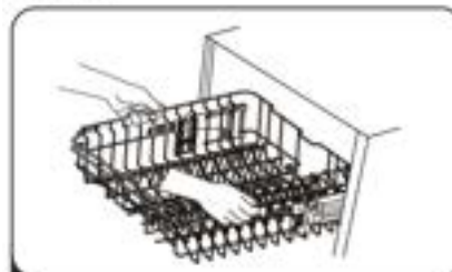
1 To raise the upper basket, just lift the upper basket at the center of each side until the basket locks into place in the upper position. It is not necessary to lift the adjuster handle.
